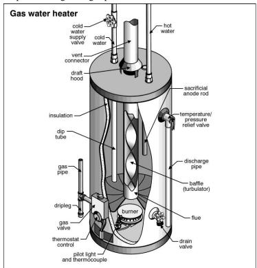
Inspect the exhaust stack on gas fired water heaters to ensure that all pipe connections are secure and free of rust, corrosion, and obstructions (annually). (**Note**: It is essential that fuel fired water heaters vent their gasses to the outside; escape of gasses inside the home could be lethal and pose a fire hazard.)
