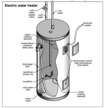
Water Heaters located in the garage or compartments opening into the garage should be mounted at least 18" above the garage floors lowest elevation. This helps protect the water heater from physical damage and helps prevent the possibility of causing fires by igniting hazardous paint, gasoline or other flammable vapors.
